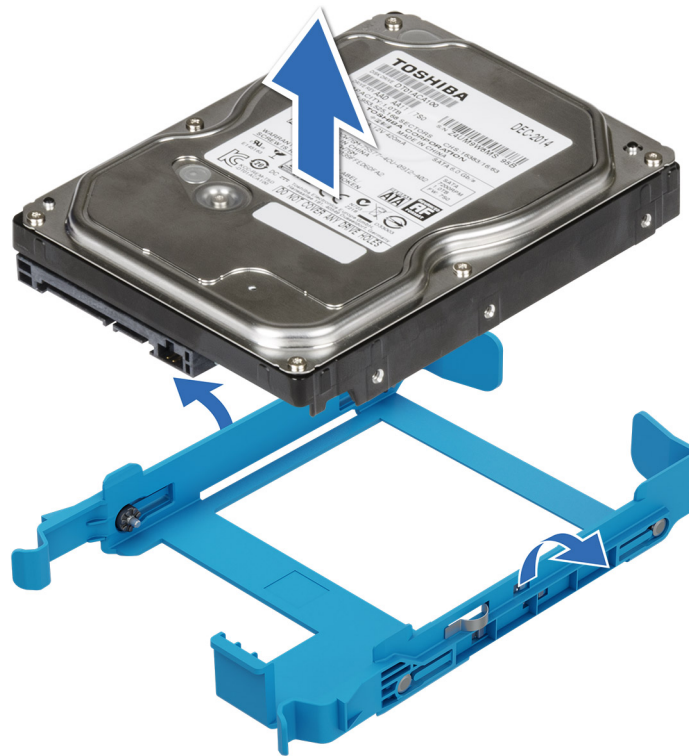
Figure 24. Removing the drive from the drive carrier
