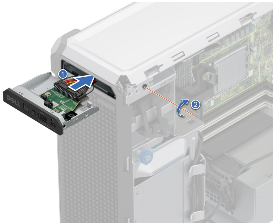
Figure 69. Installing the control panel cage
