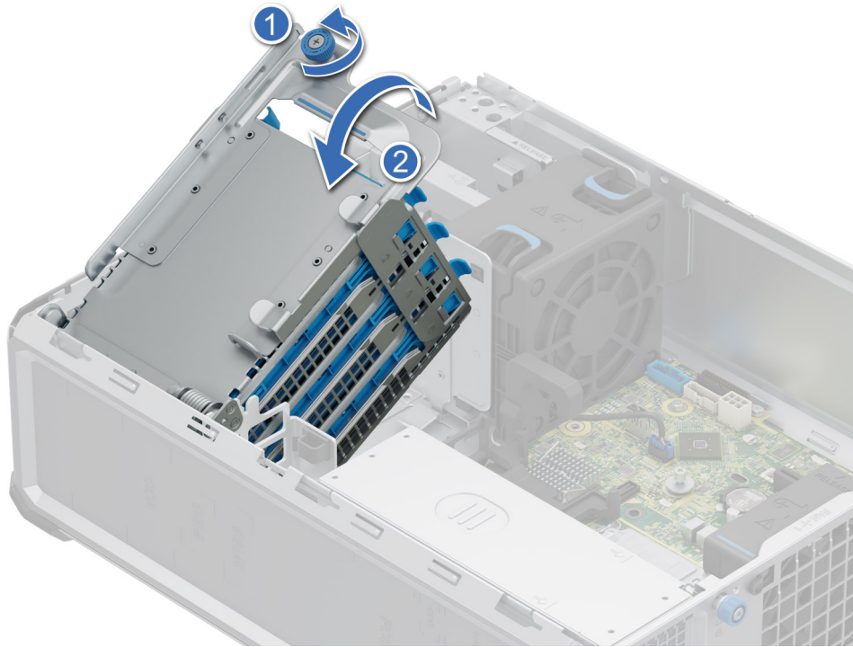
Figure 18. Removing a drive from drive cage
