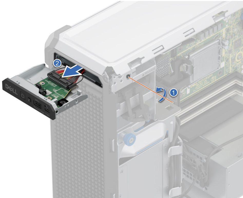
Figure 66. Removing the control panel cage
