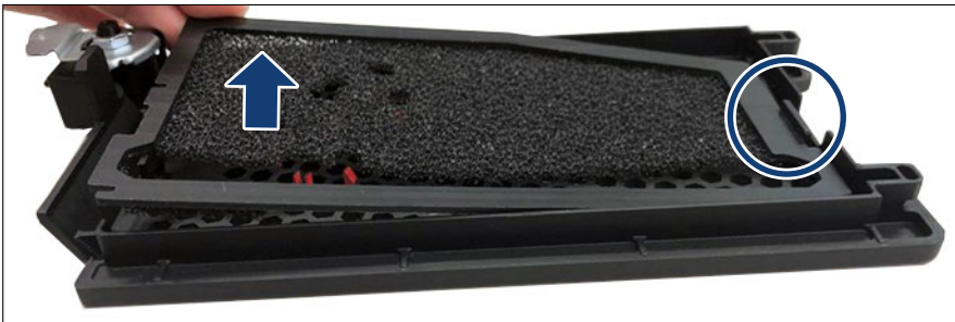
Figure 203: Removing the dust cover 1
