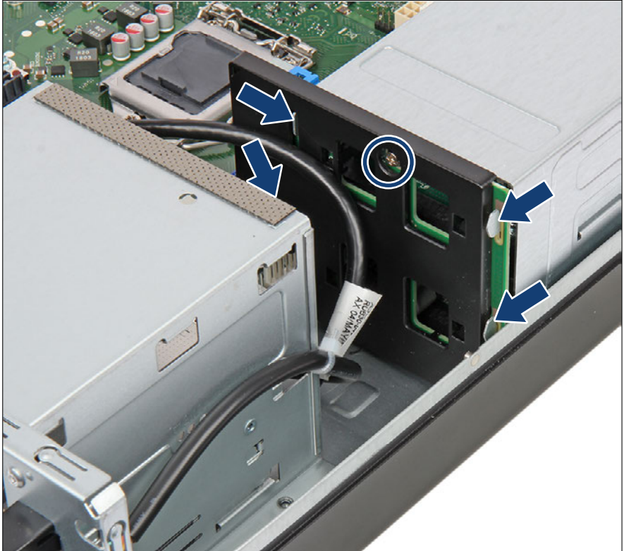
Figure 55: Installing the power distribution board
