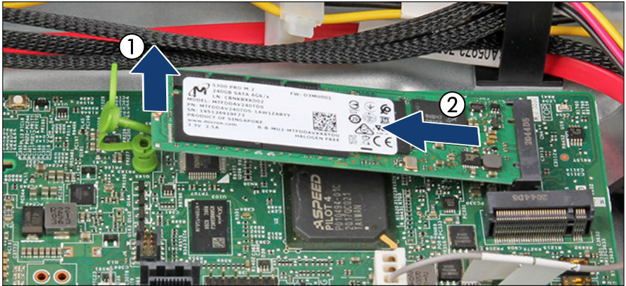
Figure 226: Removing the M.2 SSD (B)
