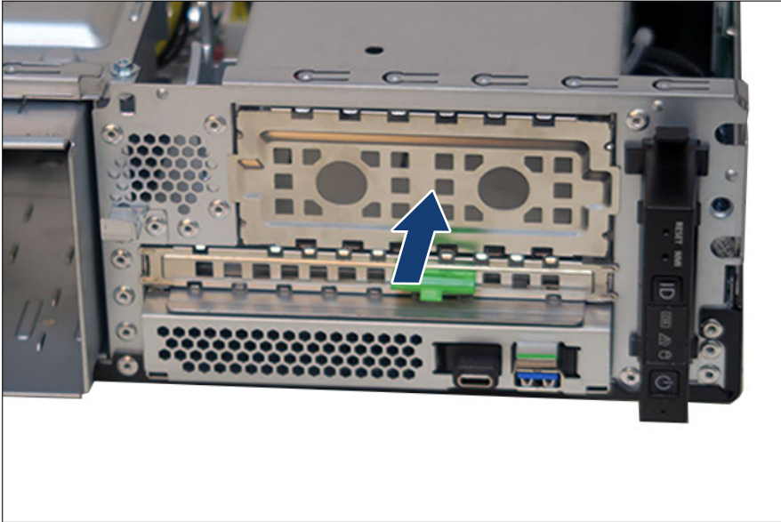
Figure 178: Installing the RDX drive filler cover
