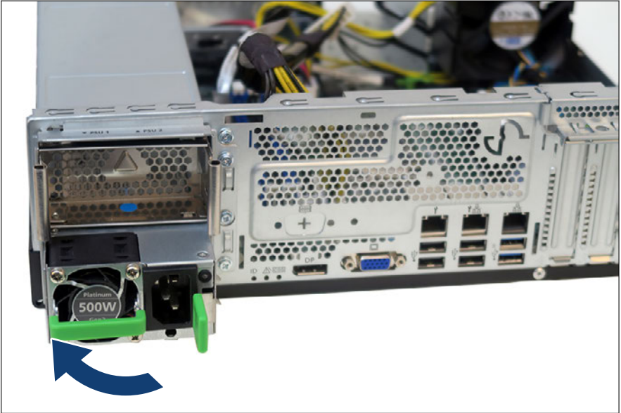
Figure 42: Folding up the handle
