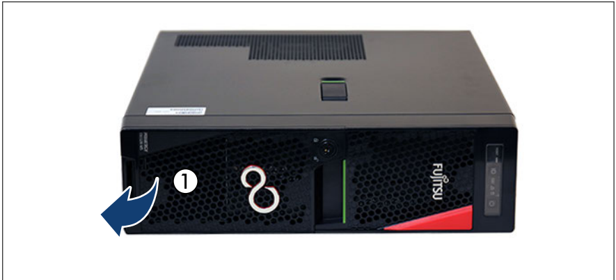
Figure 9: Removing the HDD bay cover
