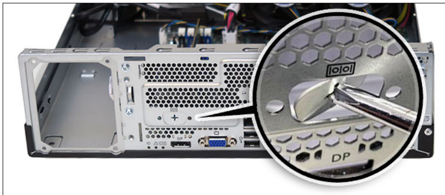
Figure 188: Removing the metal cover
