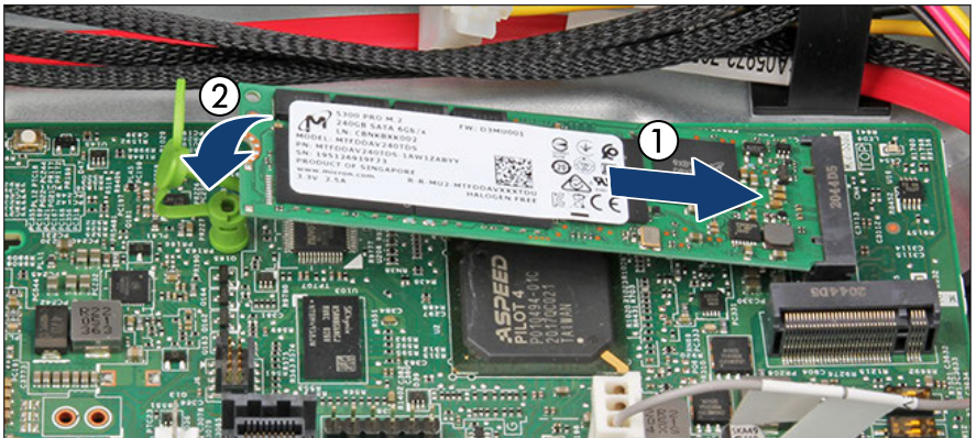
Figure 223: Installing the M.2 SSD (A)
