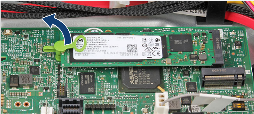
Figure 225: Removing the M.2 SSD (A)
