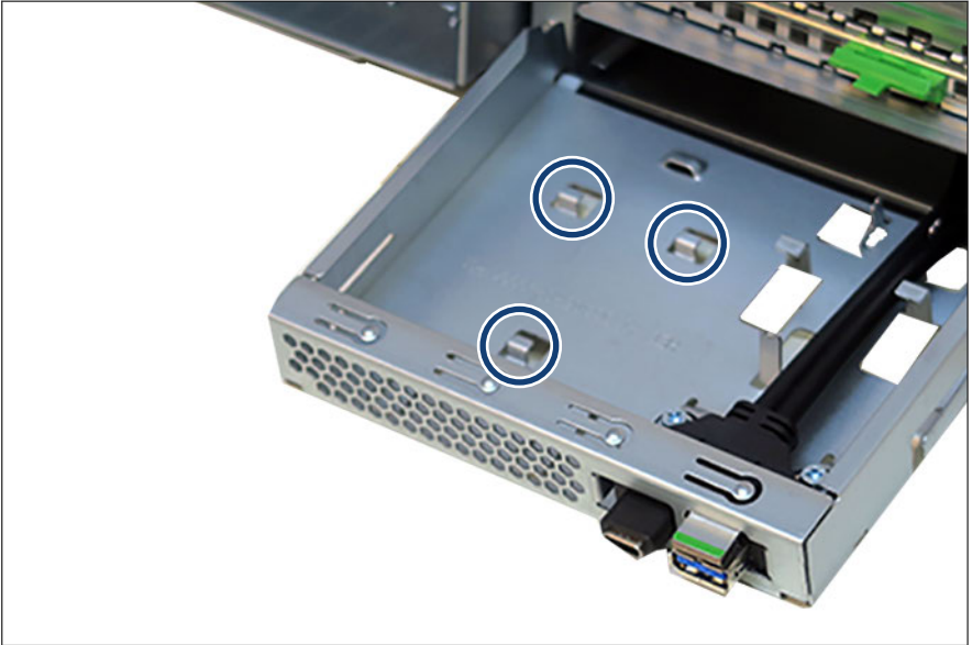
Figure 131: Hooks on the FBU tray
