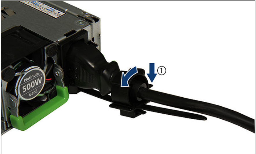
Figure 3: Unlocking the cable clamp of a PSU
