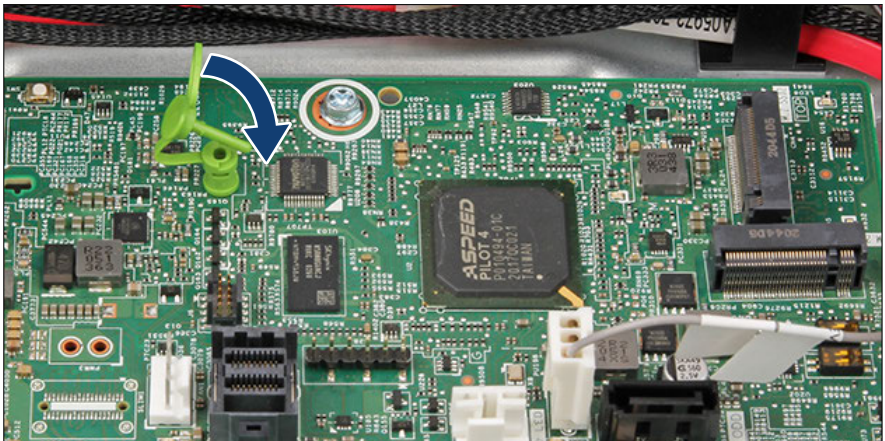
Figure 227: Closing the M.2 lock
