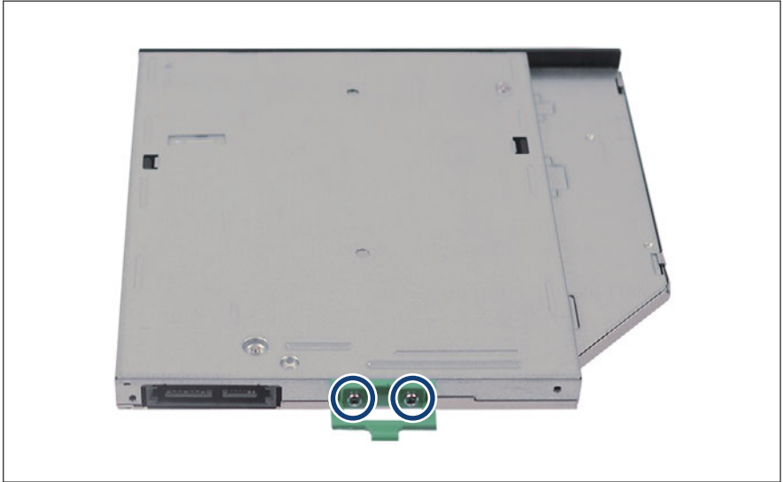
Figure 163: Installing the ODD latch on the ODD
