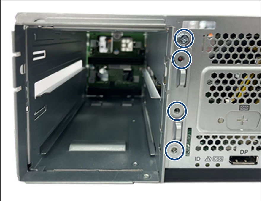
Figure 39: Fastening the redundant PSU frame
