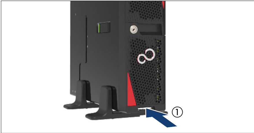
Figure 13: Installing the ID card
