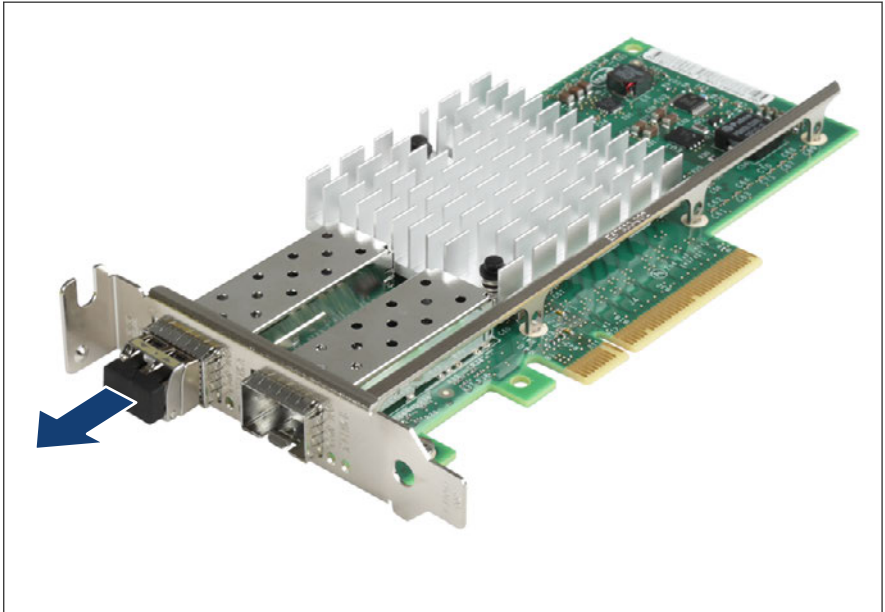
Figure 109: Removing the protective cap
