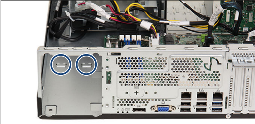
Figure 32: Hooks on the bottom of the chassis
