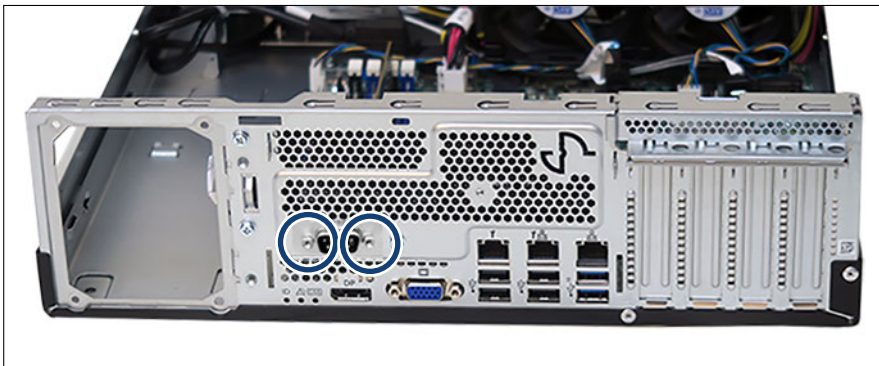
Figure 191: Removing the serial interface (A)
