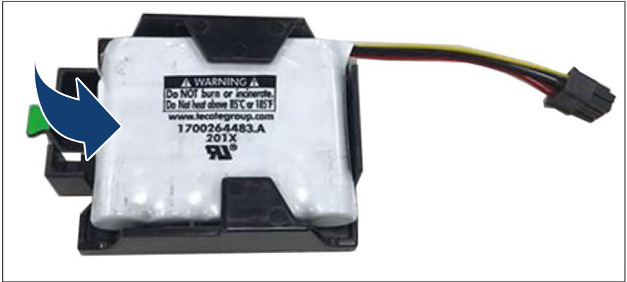
Figure 129: Installing the FBU in the holder
