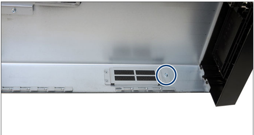
Figure 199: Installing the dust cover 4 (B)
