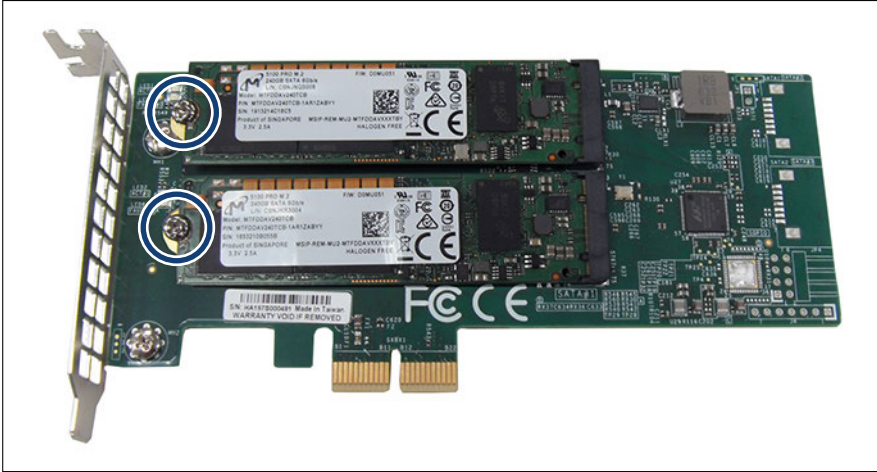
Figure 123: Installing M.2 SSDs (B)
