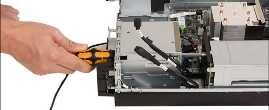
Figure 49: Access to the screw of the power distribution board
