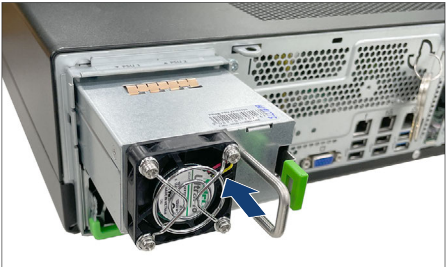
Figure 57: Installing an FJBU
