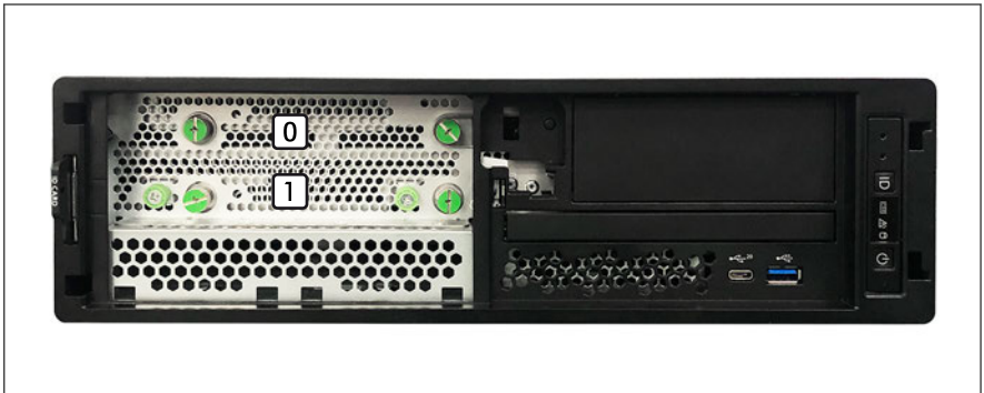
Figure 62: Configuration with up to two 3.5-inch HDDs
