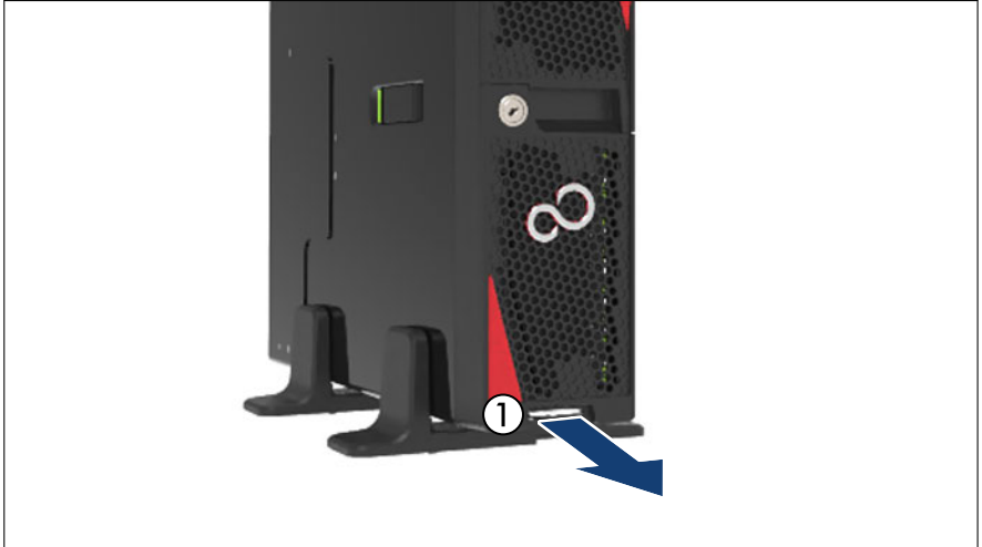
Figure 6: Removing the ID card
