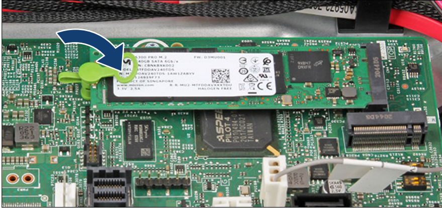
Figure 224: Installing the M.2 SSD (B)
