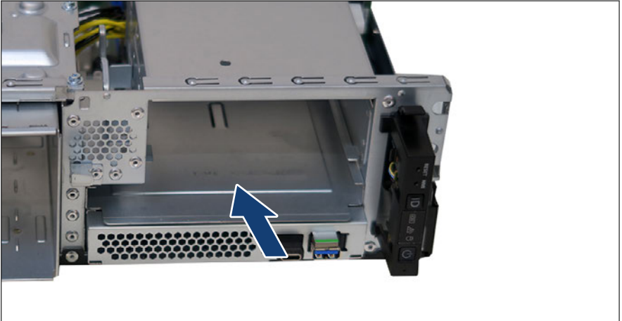
Figure 138: Installing the FBU tray
