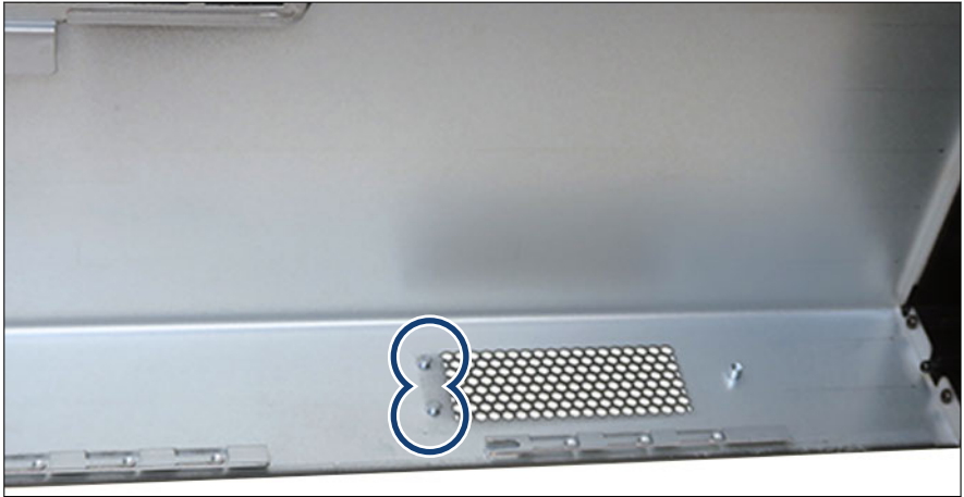
Figure 198: Installing the dust cover 4 (A)
