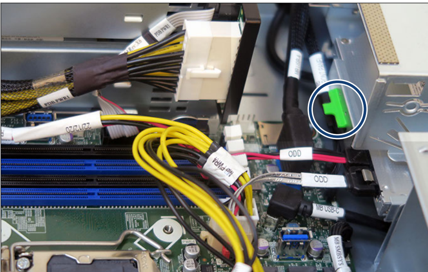
Figure 165: Installing the ODD (B)
