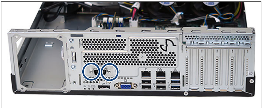
Figure 190: Installing the serial interface (B)
