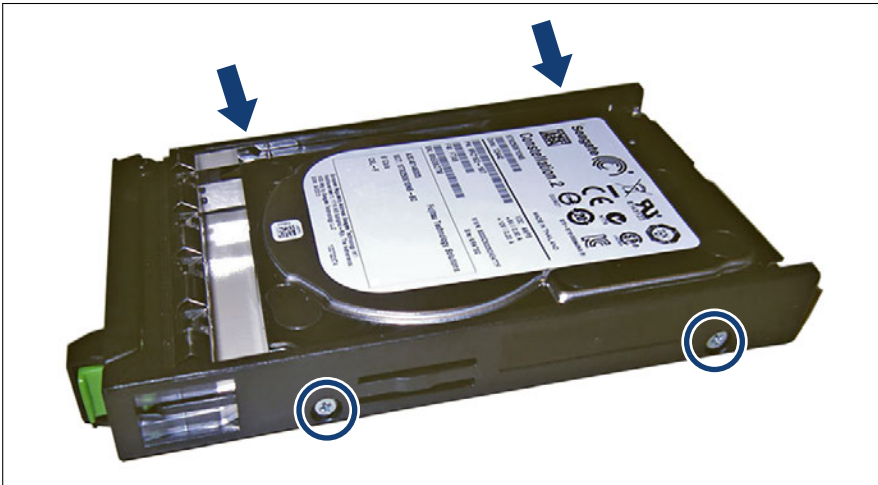
Figure 61: Installing the 2.5-inch HDD/SSD in the 2.5-inch installation frame (B)
