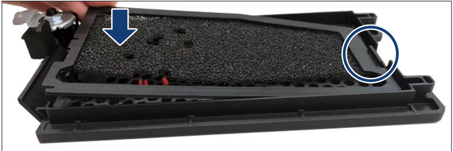
Figure 194: Installing the dust cover 1
