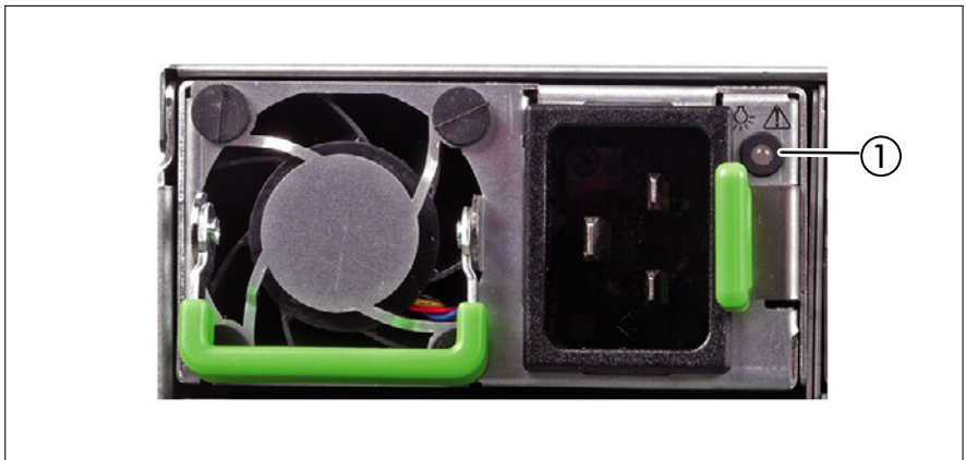
Figure 253: Indicator on hot-plug PSU
