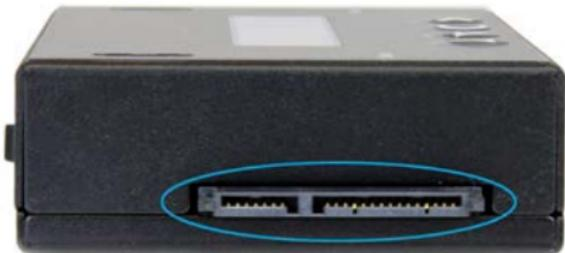
3. Connect your **Target drive** to the **SATA SSD/HDD Target Port** on the **SATDUP11IMG**.
