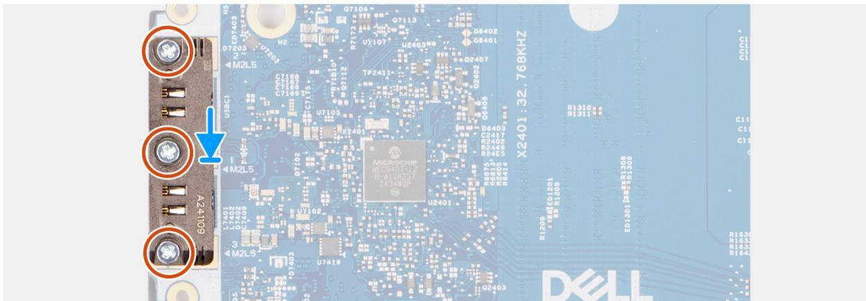
**Figure 49. Installing the USB Type-C module**
