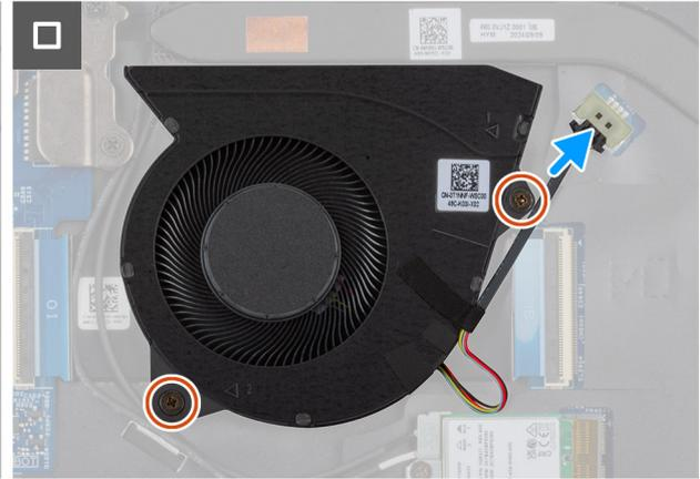
**Figure 31. Installing the fan**
