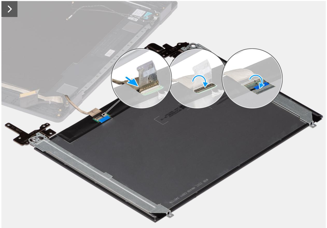
Figure 79. Installing the display-panel assembly
