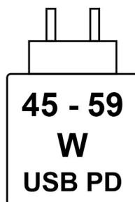
**Figure 8. Pictogram for power charging requirements**
