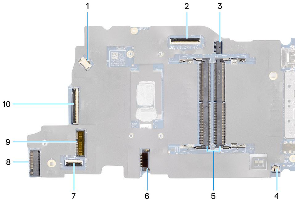
**Figure 42. System-board connectors**
