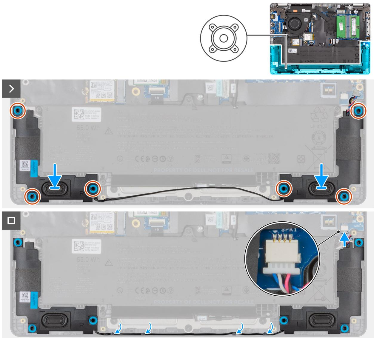
Figure 28. Installing the speakers
