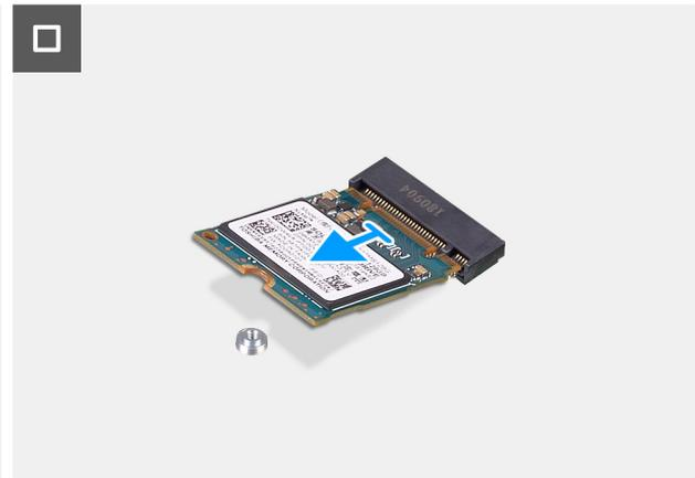
**Figure 23. Removing the SSD**
