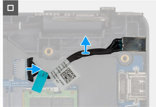
**Figure 32. Removing the power-adapter port**
