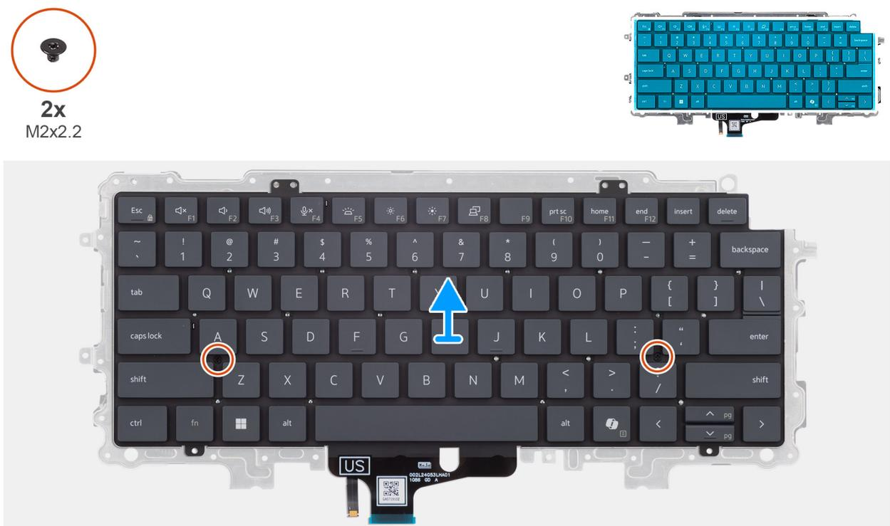
Figure 56. Removing the keyboard support plate
