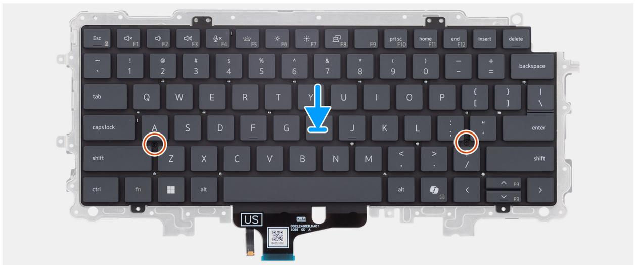
Figure 59. Installing the keyboard support plate
