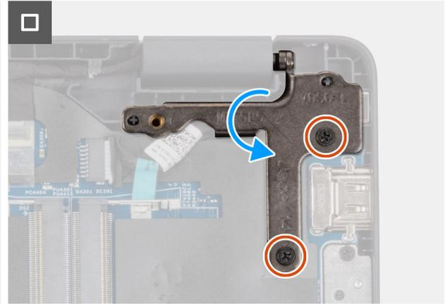
**Figure 33. Installing the power-adapter port**
