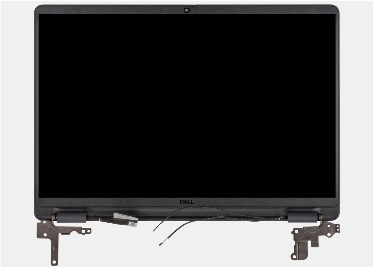
Figure 64. Removing the display assembly
