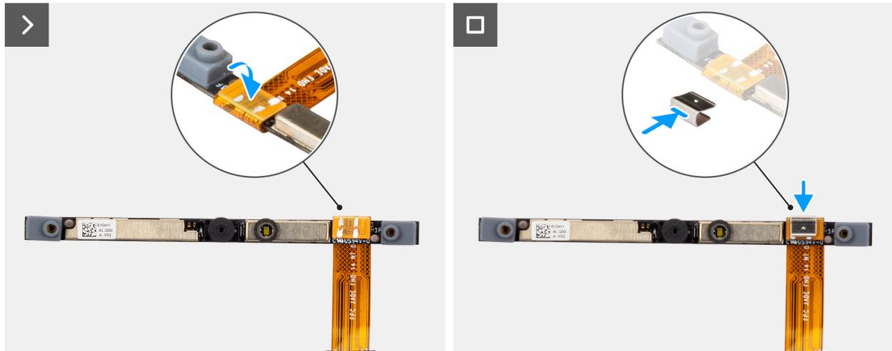
**Figure 83. Installing the camera**
