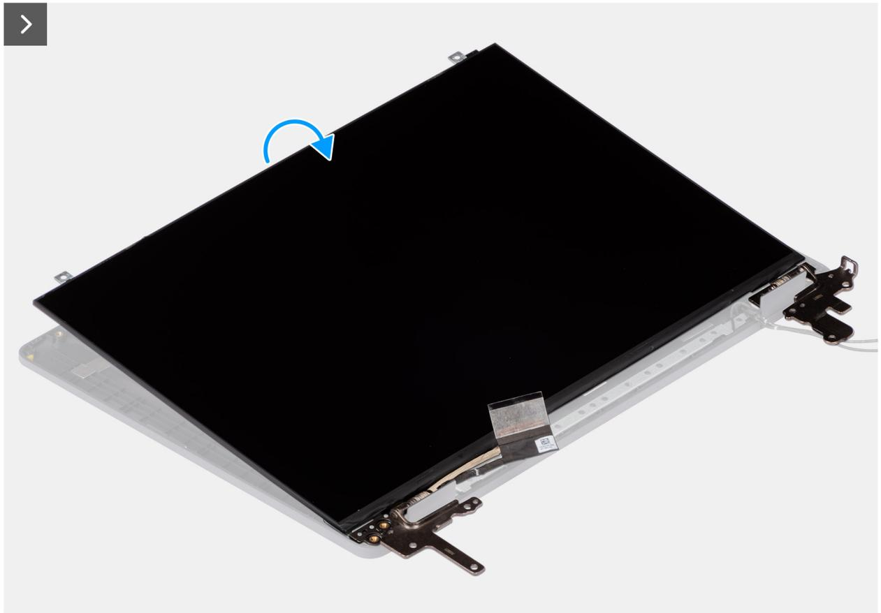
**Figure 75. Removing the display-panel assembly**
