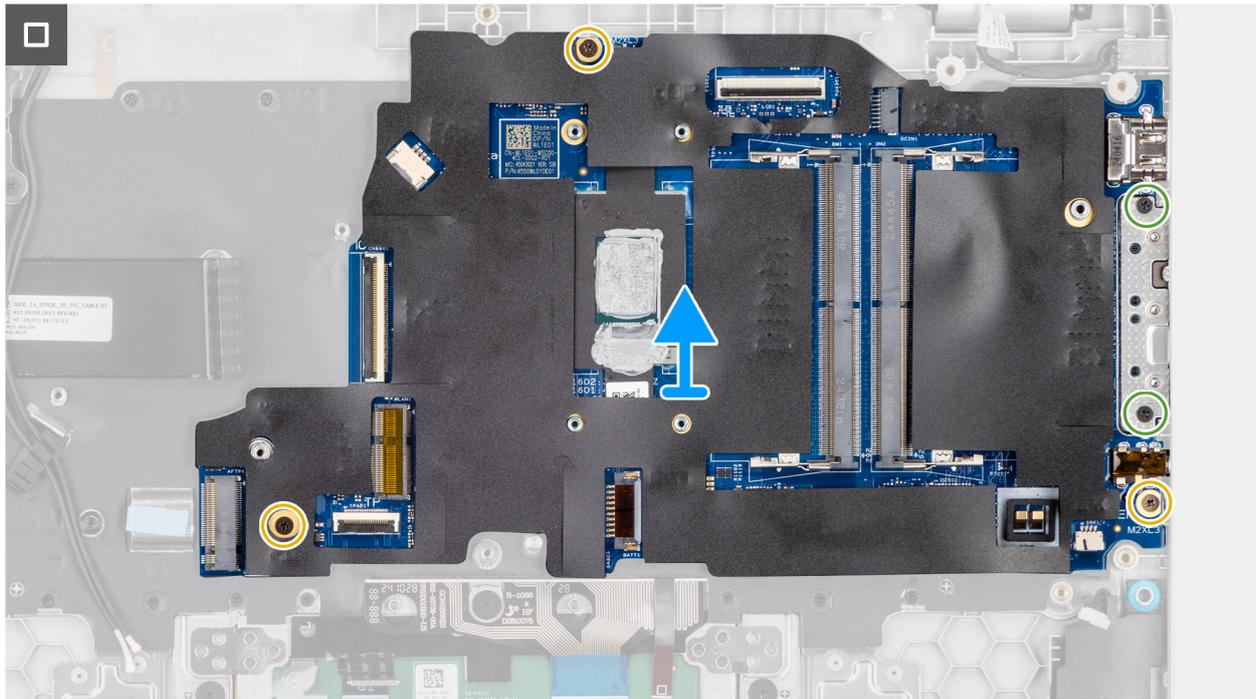
**Figure 44. Removing the system board**
