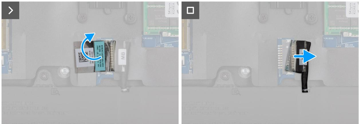
Figure 13. Disconnecting the battery cable
