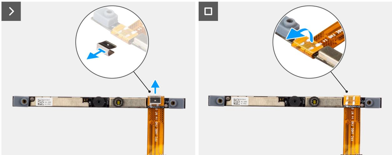
**Figure 82. Removing the camera**
