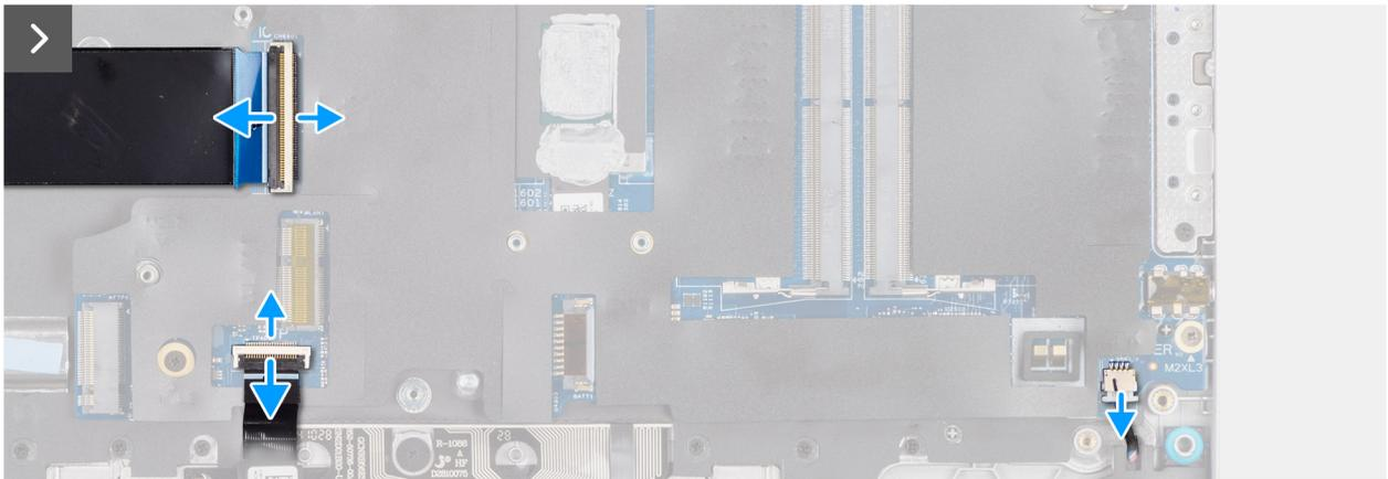
Figure 43. Removing the system board
