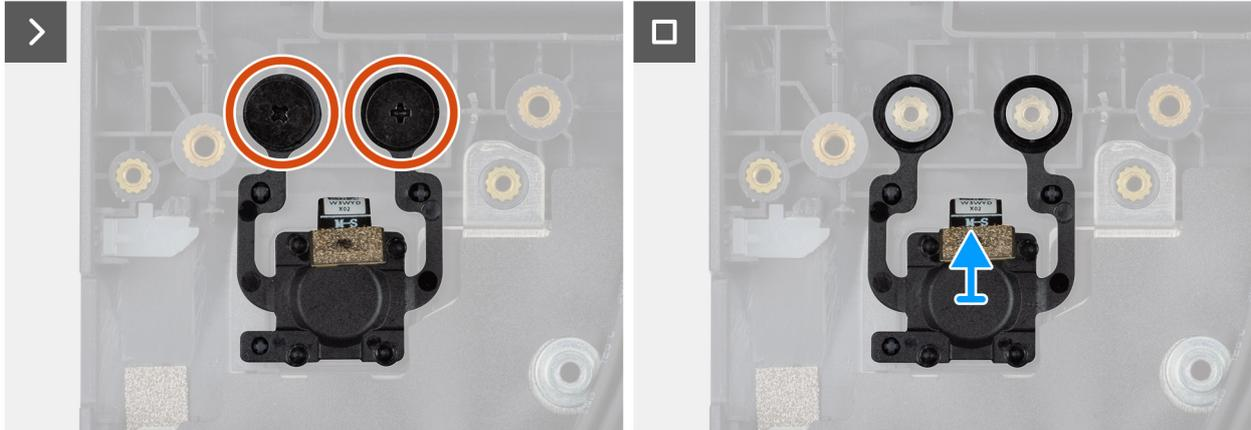
Figure 40. Removing the power button with fingerprint reader
