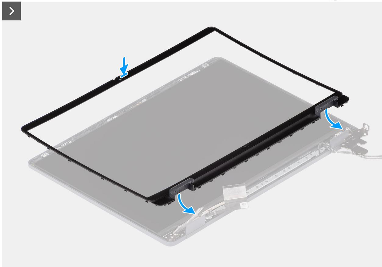
Figure 72. Installing the display bezel
