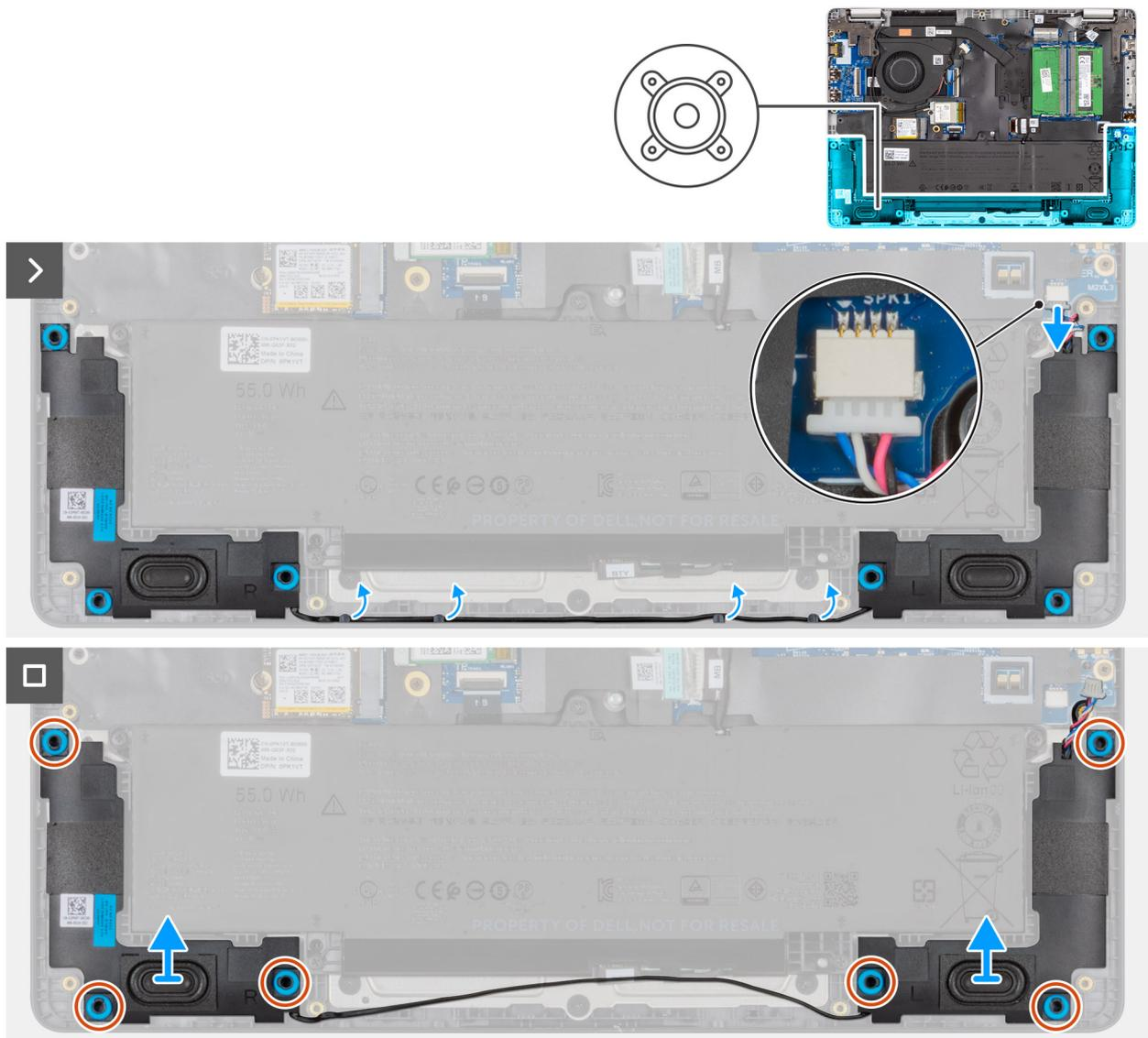
Figure 27. Removing the speakers
