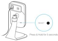
While the camera is powered on, press the **RESET** button for **5** seconds until the System LED on the front panel turns solid red. The camera will reset and reboot.
