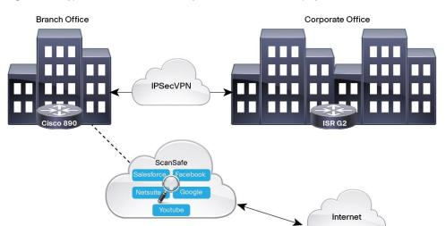
Figure 3. Typical Cisco ISR Web Security with Cisco ScanSafe Deployment
