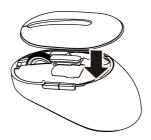
**5.** Slide the power switch down to turn on the mouse.
